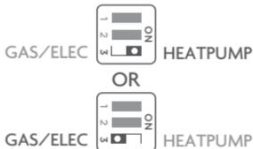
This dip switch configures the thermostat to control a conventional gas/electric system or a heat pump. If your system is anything other than a heat pump, leave this switch set for **GAS/ELEC**.
